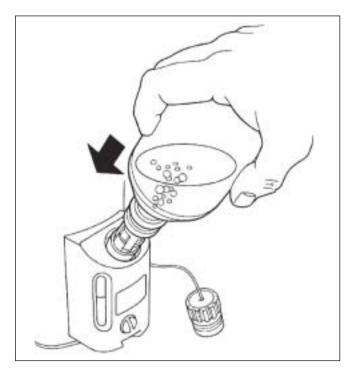
Figure 2 –Key-Indexed System for Inhalational Agents. The illustration of the Delta Vaporizer, Quick Fill type, was reproduced with permission of Penlon Ltd, Abingdon, UK.
